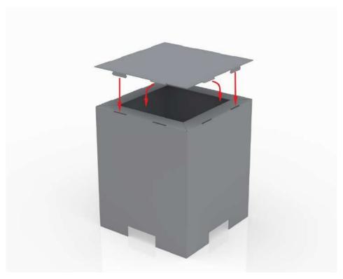
D. Place the box over each STOPPER ensuring that the cable runs through the bottom cable cut-outs and sits flat on the floor.
